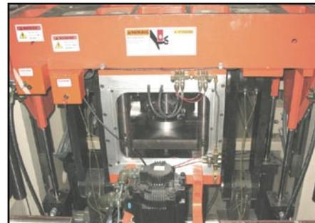
*Fig. 1. Bottom platen with plug assist servo motor in the foreground.*
